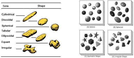
Particle shape and size plays a significant part in the bulk density of a product. The more uniform and cubic the particle shape, the lower amount of gaps there are between the particles and therefore the less amount of gas. Particle shapes can be:-
