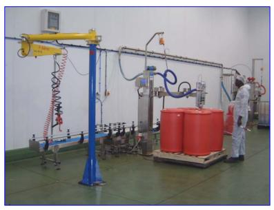
The Weightron Bilanciai system is based around a gravimetric StrongArm filling machine, which offers significant flexibility and versatility. The Healy Group's Mervyn Operations Manager Penson is very upbeat about the new system and as he explains: "The design of the line gives us the best of both worlds and allows us to accommodate the different filling requirements for the wide range of end customers. The
