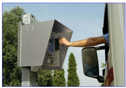
and tare weight. Using this information, the terminal then issues a ticket showing the calculated net weight of material being collected (or delivered), thereby removing the need for a second weighing.
