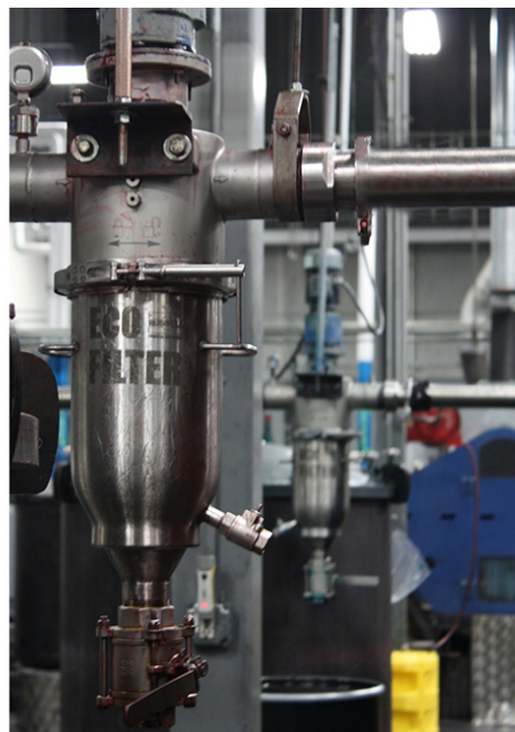
Figure 1: The Eco Filter integrates into existing pipelines to remove metallic contamination
