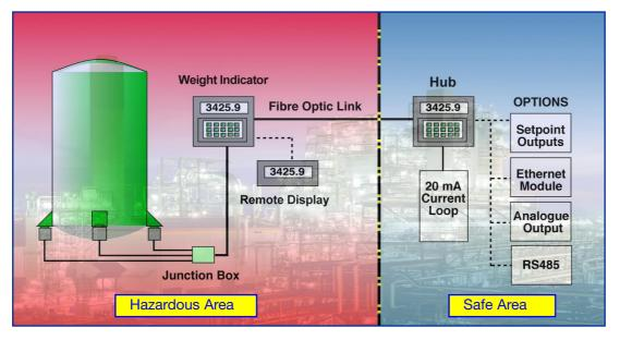
This third example shows a fibre optic link between the hazardous area and the safe area. Full functionality of the ATEX certified Weight Indicator is available via the Hub Terminal in the safe area. An extensive range of control and communication options complete flexible versatile and installation. Power to the instrumentation in the hazardous area may come from certified batteries or mains supply.
