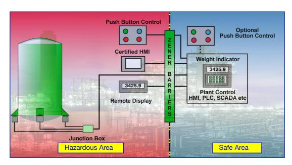
In this conventional hazardous area weighing application, the system integrity is maintained via Zener Barriers. Optional ATEX certified equipment such as remote weight displays or HMIs can be located in the hazardous area, powered from the safe area via the Zener Barriers. Control functions can be carried out in either the safe or hazardous area.
