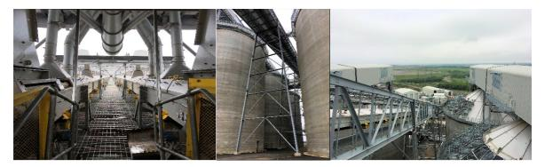
As will be noted, and expected, each of the main storage silos are fitted with explosion panels and slam-shut valves to protect the silos and their contents. Once having been extracted at a controlled rate from the main storage silos the biomass fuel pellets are, once again, transported to the intermediate silos by a twin, air supported, belt conveying system.
