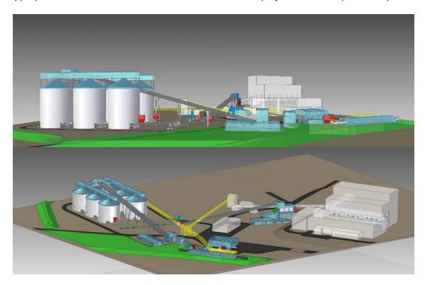
In order to ensure security of supply Lynemouth is able to accept biomass fuel by two means — rail and road. Rail is the predominant means of delivery and the station is provided with biomass wood pellets by a dedicated rail spur that can receive up to four 2,000t trains a day from a specialised bulk store constructed at Port of Tyne. As will be observed from the following photographs adjacent to the rail unloading facility are three road vehicle unloading stations.
