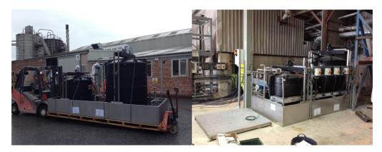
The complete dosing skid was manufactured in a standalone bund to enable ease of installation and testing and prewiring of major components. Tank levels were monitored by means of load cells to cross check dosing rates and continuously monitor levels to allow complete automation and a effectively provide a continuous dosing unit from a batch make up system.
