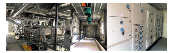
The drag link conveyors and screw conditioners and screw conveyors have been provided by Fairport Engineering's sister company Fairport Process Equipment Ltd. Recently completed after a six month construction period the conditioning facility is currently being commissioned.
