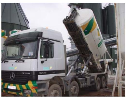
A mobile DSM silo being loaded for delivery to site
