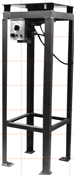
FT 18" x 18" x 44" table with a variable high frequency vibrator for the making of molds for precision castings used in orthopedic surgery, such as hip joints, etc. Height was determined by a stationary microscope under which the work was done.
